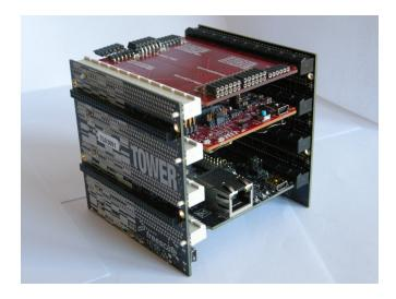
Don't care slot position, but be careful to connect Primary and Secondary connector properly. Take care at reference signed near PCI board connectors.
